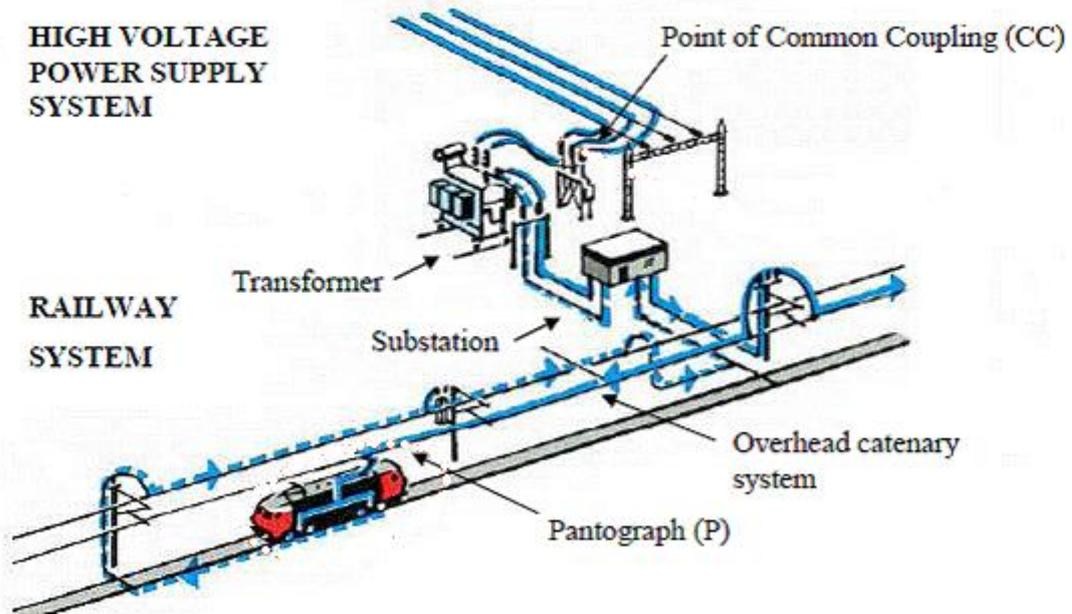
Fig. 4: Railway System and position of the Substation
