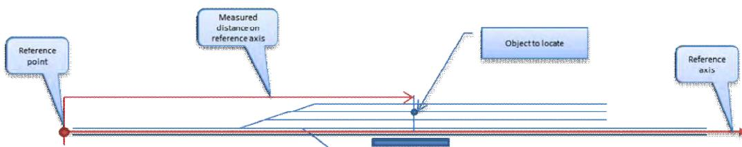
*Traditionally, the reference axis is the railway LINE, and the distances are measured from reference points on the field (mileposts)*
